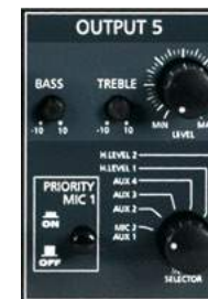
Individual controls on each channel. Tone control, gain, input source selection and implementation of priority microphone.
