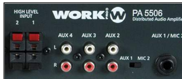
Rear input connections: Mic, Aux and high level inputs (HI-LV).
